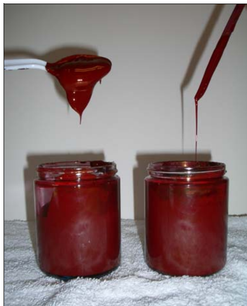
Esperse 506 provides a highly flowable dispersion with high pigment loading, as seen on the right. A competitive product, on the left, produced a highly viscous and pseudoplastic dispersion at equal pigment loading.
